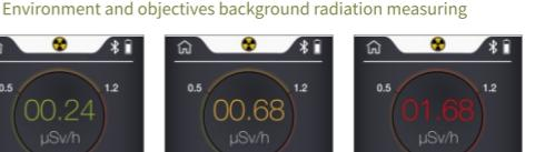
Greentest Eco starts measuring the background radiation immediately after the device is turned on. The result of the ionizing radiation test is displayed and a recommendation is issued.
